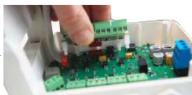
Place the relay module by matching the holes for spacers (1 on previous picture) and the red connector (2 on previous picture).
